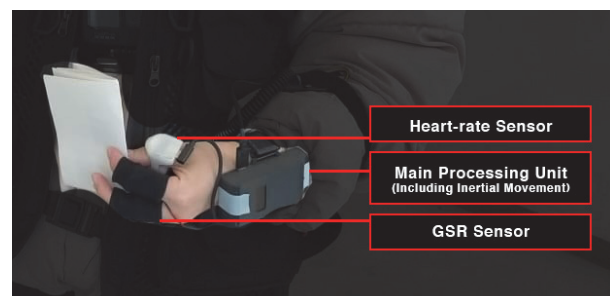
Fig. 2. My Daily Badge was used to capture the biometric data via a heart-rate sensor, GSR sensor, and inertial movement (Onchi et al., 2021)
