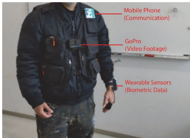
Fig. 1. Participants were attached with sensors for biometric data (left wrist), camera for video footage (chest), phone for communication (left shoulder)
